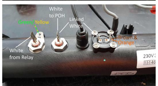
Titanium Heater Element post Nov 2015 wiring connections
