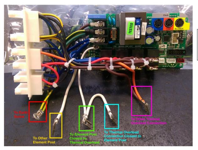
SP601 circuit board V8 with post Nov 2015 wiring loom
