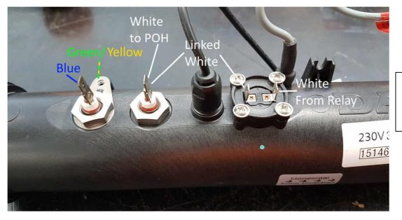
Titanium Heater Element pre Nov 2015 wiring connections
