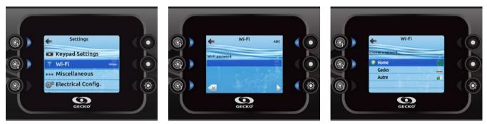
For the Wi-Fi menu to appear in the Settings menu your in.touch module must be equipped with software version 11.00 or higher. This menu allows you to connect your in.touch module to a Wi-Fi network or to change its network.
