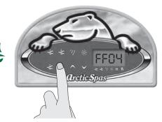
Press the filter cycle key again to display the number of cycles (FF) in a 24 hour period. You can select from 1 cycle to 4 cycles per day. The Filter Cycle triangular icon will appear on the display when a filter cycle is on.
