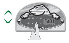
Use the Up & Down arrow keys to change the number of hours. 00 = no filtration 01 = 1 hour/cycle 02 = 2 hour/cycle
