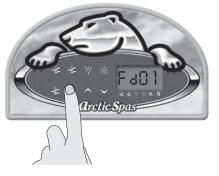
Press on the Filter Cycle key. The display will show Fd XX where XX represents the number of hours Pump 1 will be operating at low speed.
