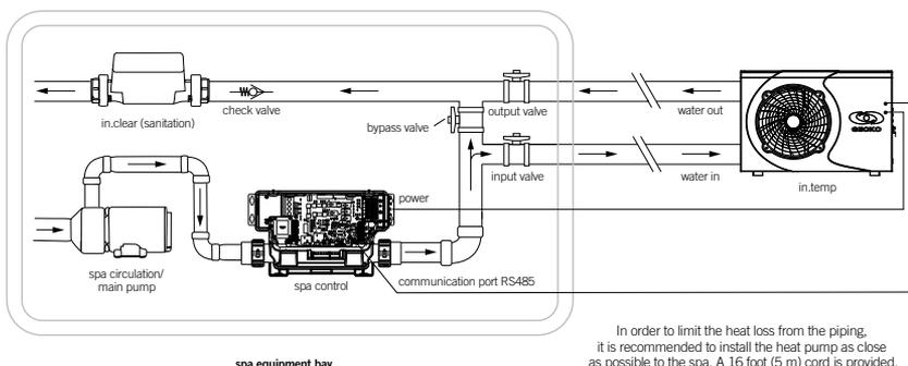
In order to limit the heat loss from the piping, it is recommended to install the heat pump as close as possible to the spa. A 16 foot (5 m) cord is provided.
